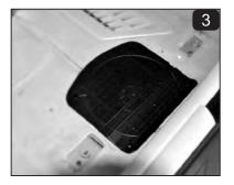
Factory subwoofer is under the cover, ready for the CDT BM8-Sub1 installation.
