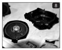
In case of the factory subwoofer is glued, be careful not to damage the plastic enclosure which can be re used for the CDT BM8-Sub1.
