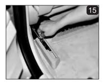
Firmly tighten the "front" and "rear" screws of the seat track
