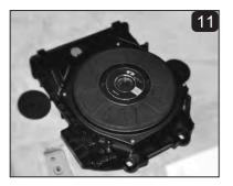
Replace the factory subwoofer by CDT BM8-Sub1 and re tighten the screws.
