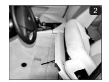
After the screws removal, tilt down the seat to provide access to the subwoofer replacement.
