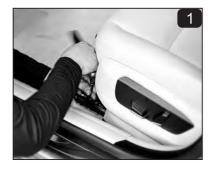
Remove the screws that hold the driver's seat track to the floor.
