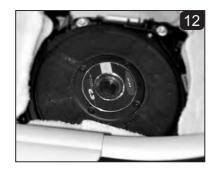
Once you have mounted the subwoofer into the plastic enclosure securely, re install the subwoofer into the floor pocket.
