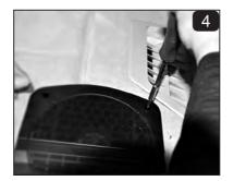
Loosen the factory fixed screws of the subwoofer cover.
