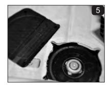
Once all the fixed screws are loosened, remove cover to expose facorty subwoofer.
